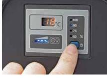
Automatic control unit: The control unit not only shows the current status of your lamps and the water temperature, it also allows you to adjust the output to suit your needs.
