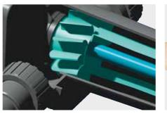
Automatic cleaning rotor: Due to the water flow, the cleaning rotor is continuously guided around the quartz glass tube and therefore prevents dirt deposits.
